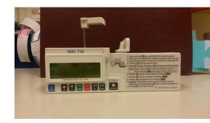
5. Load the primed syringe into the Syringe Driver BUT make sure the plunger is secure between the prongs of the plunger and the Carriage. You will feel a click(Do not force the syringe into place)
